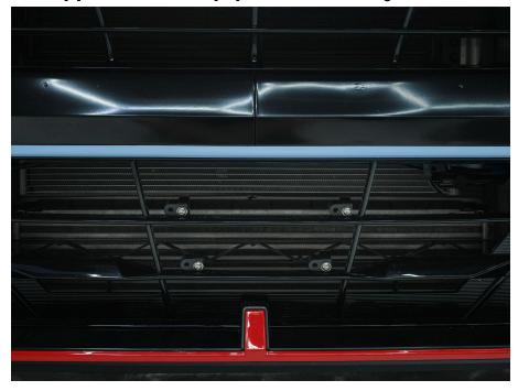
2. Clamp the wedge clamp assemblies to the grille. Refer to the above photo for a reference for the positioning. The bottom of the clamp needs to fit into the gap of the grille slots.
