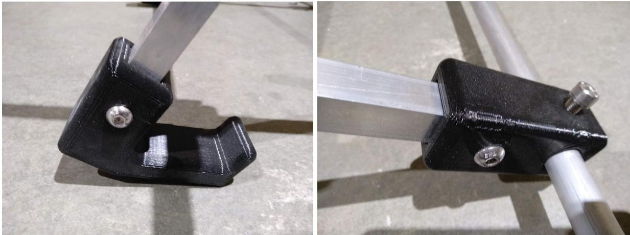
Assemble your rods onto the 3-way blocks and test fit on the vehicle and you can mount the strings to your alignment kit to see how it all fits. Use the thumb screws to lock the string holder rod and 3-way blocks in place. Once you've set up the string and decided where all your bars should go, it's nice to mark the tubing with a marker so you can quickly dial it back in if the kit gets disassembled for transport or other cars.
