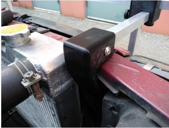
Measure how long the bars for the chassis hooks should be to clear the bumper. Usually 40-60cm is sufficient.
