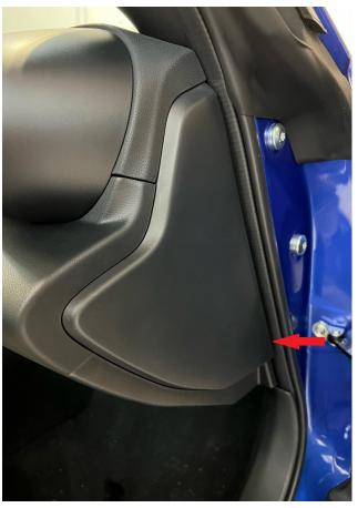
3. Secure OBD port by reusing the screw in the inboard side of the glovebox cavity.
