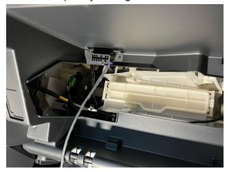
4. Use the provided screw to secure the other side of the OBD port to the glove box
